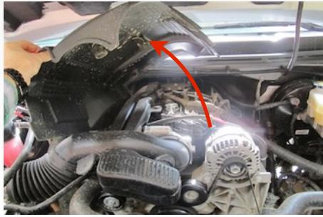
3. Disconnect the crank case vent line from the intake tube plenum by gently pulling it out.
