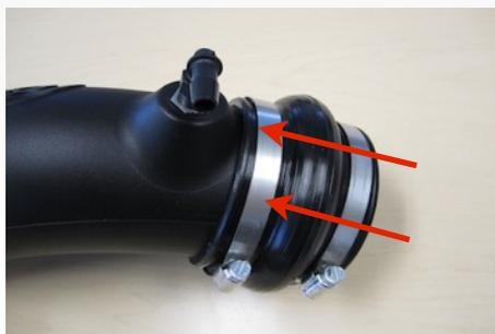
20. Secure the Silicone Step Coupler (S) to the throttle body using a #64 Hose Clamp (M). Place the #72 Hose Clamp (R) around the top of the Silicone coupler.
