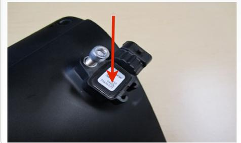
15. Remove the MAF sensor from the OE air cleaner using the supplied T15 Torx key. Install it into the Filter Adapter Tube (K) using the supplied 8-32x1/2" Screws (J). Do not over tighten.
