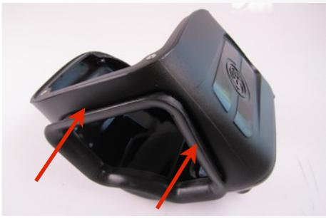
13. Install the Air box assembly using the supplied M6-1.0x10mm Screws (T) and 6mm Washers (U) in the two holes closest to the fender and the 2 longer OE screws in the remaining two holes.
