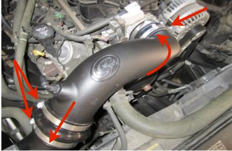
22. Push the Silicone Breather Hose (Q) over the Hose Barb (P) on the Intake tube. Then push the other end onto the valve cover vent line. Trim hose to desired fit if necessary. Hose should not be resting on other parts.
