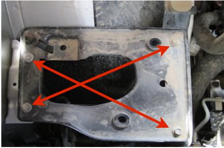
11. For those concerned about minimal engine heat; install the Air Inlet Plug (A) into the bottom of the Air Box (B) by pushing it down until the bead catches the lip as shown below. For those seeking additional air flow, set the Air Inlet Plug aside. (See page 3 for more info and test results)
