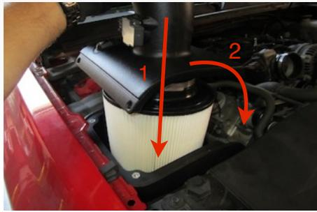
17. Install the Clear Lid (H). Secure the Lid and Filter Adapter using the supplied 1/4"-20x1-1/4" S.S. Screws (I) and Rubber Washers (F). Then use the 1/4"-20x5/8" S.S. Screws (G) and Rubber Washers (F) in the remaining two holes.
