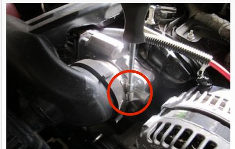
7. Disconnect the intake tube from the air cleaner assembly. Then remove the intake from the vehicle.
