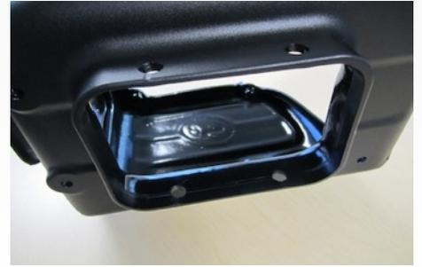
12. Install the Air Inlet Fender Seal (C) onto the lip of the Air Box (B).
