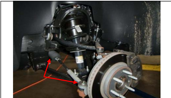
Photo shows inner/outer tie rod assembly
