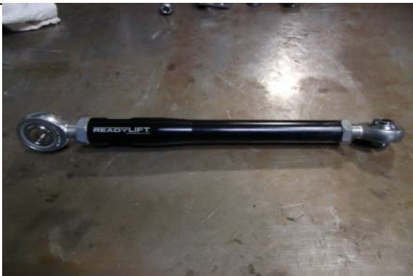
Picture of assembled steering assembly
