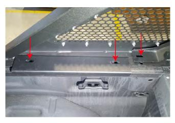
**STEP 8**// Once the rack is aligned as desired, place the bed rail plates on top of the chase rack. Mark the (3) 1/2 inch hole locations. Drill through your factory bed rail and insert the (6) M12 bolt plates, lock washers, and flat washers securing the chase rack to the bed frame. Repeat on other side.
