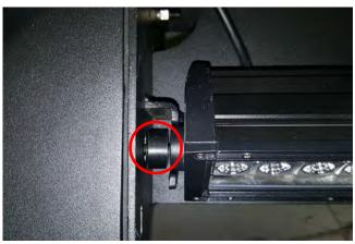
**STEP 9**// Light bar must be installed prior to installing the upper mesh cover. Insert the M8 x 40mm bolts, lock washers, and flat washers through the upright and light tray. Install the provided spacers between the light bar and the tray as seen above. Do to the differing widths of 40" light bars, additional 2.5mm spacer/washers are included.
