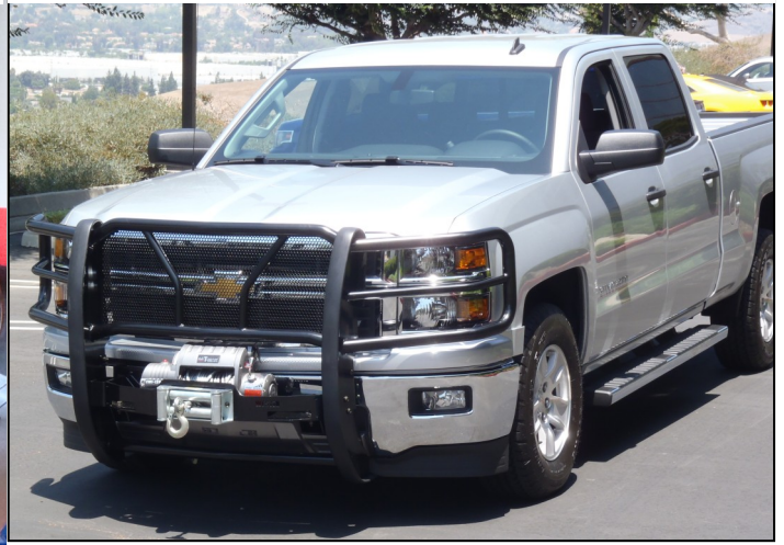
HDX Winch GG Installation Complete
