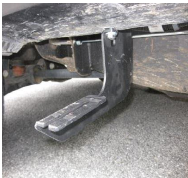
2) Insert M8 Unut on vehicle as shown above
