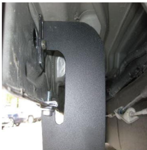
1) Insert M8 Unut on vehicle pinch weld
