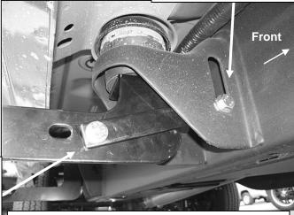
(Fig 9) Example of passenger side, 1500 Model Center Bracket and Support Bracket Installation
