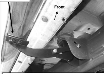
(Fig 13) Passenger side Center Bracket Installation
