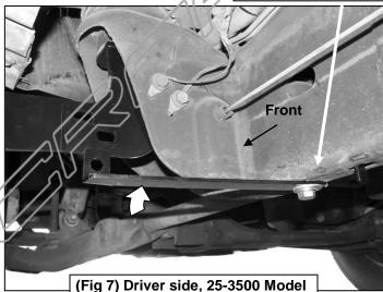
Front Support Bracket Installation
