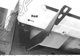
(Fig 11) Passenger side Rear Bracket Installation
