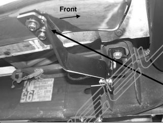
(Fig 12) Passenger side Front Bracket Installation
