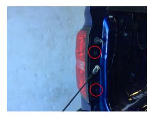
**Step 2:** Twist the bulb sockets to remove the tail light harness from the light.
