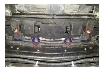
**STEP 3** // From underneath the vehicle, remove the lower (4) 10mm grille bolts. Remove grille completely.
