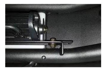
**STEP 10** // The bumper will include a bolt on mesh cover. Secure the cover to the bumper using (4) M8 x 20mm bolts, lock washers, and nuts. If purchased with the LED lighting option: Install the LED light using the hardware provided in the light packaging.
