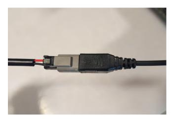
**STEP 13** // Optional LED Wiring: Connect the supplied wiring harness to the LED lights. Be sure to zip tie the excess wiring away from hot/moving engine bay components.
