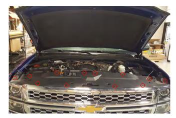
**STEP 1** // Using a panel removal tool, remove the (12) plastic grille cover push pins and remove the grille cover.
