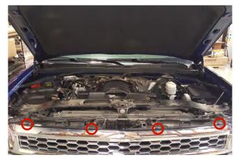
**STEP 2** // Next, remove the upper (4) 10mm bolts holding the grille in place.
