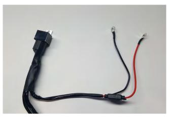
**STEP 14** // Optional LED Wiring: Install the Red 12+ volt wire to the positive battery terminal. Connect the black ground wire to the negative battery terminal. Secure any excess wiring away from any hot/moving engine bay components.
