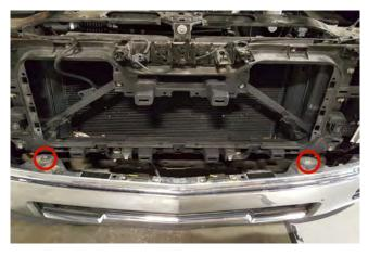
**STEP 5** // Remove the (2) 21mm bolts on top of the bumper that hold it to the bumper brackets. Remove bumper.
