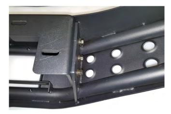
**STEP 7** // Install the (2) new bumper brackets to the Barricade bumper using the (3) M10x1.50x35mm bolts, flat washers, lock washers, and nuts per side.
