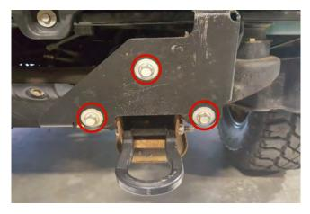
**STEP 6** // Remove the (3) 21mm bolts holding the factory bumper brackets to the frame. Remove the bolts from the other side and remove the brackets. If equipped, remove the tow hooks, they will be reinstalled in step 9.
