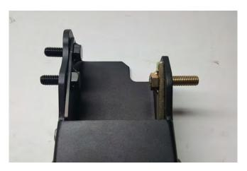
**STEP 9** // Tow hook extension bracket install: Insert the double bolt plate, and single bolt plate in the tow hook brackets as shown above and install in the factory location using the (3) M12 flat washers, lock washers, and nuts.
