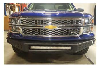
**STEP 11** // Slide bumper into place, and secure using the factory hardware.
