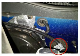
**STEP 15** // Optional LED Wiring: Route the on/off switch to the interior of the vehicle using a suitable body grommet. Mount the switch in the desired location. Safely secure any excess wiring out of the way.
