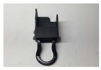
**STEP 8** // If equipped with factory tow hooks, use the factory hardware to install the tow hooks to the extension brackets.
