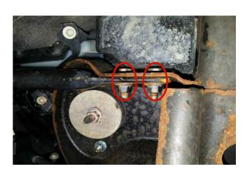
**STEP 4** // From underneath the vehicle, remove the (2) M10 bolts holding the front bumper to the frame.
