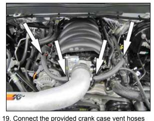
to the ports on the valve covers and then connect the open ends to the fittings installed into the K&N® intake tube.
