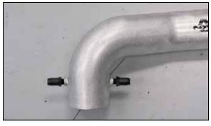
17. Install the two provided crank case vent fittings into the K&N® intake tube as shown.
