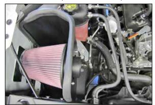
11. Install the filter assembly into the heat shield filter top first, then rotate the filter and pass the adapter through the hole in the heat shield. Secure the filter adapter to the heat shield using the provided hardware
