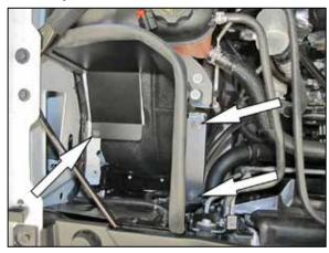
9. Install the heat shield assembly and secure the air box mounting plate location using the three factory bolts from step #7.
