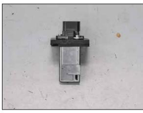
17. Install the mass air sensor into the K&N® adapter and secure with the provided hardware.
