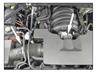
4. Loosen the two hose clamps securing the intake plenum to the factory air box and to the throttle
