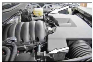
3. Disconnect the two crank case vent tubes from the intake plenum.
