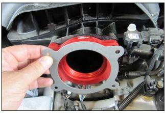
3. Install the Poweraid Spacer into the intake manifold with the supplied gasket on the throttlebody side, as shown. \*Note: Poweraid spacer must be installed with bore protruding into intake manifold away from throttle body. Incorrect installation will hinder performance. Reference picture below for spacer orientation
