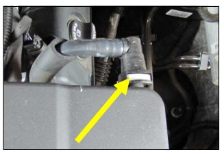
2. The quick connects for the valve cover breathers are removed by depressing the grey locking tab in the fitting and sliding them away.
