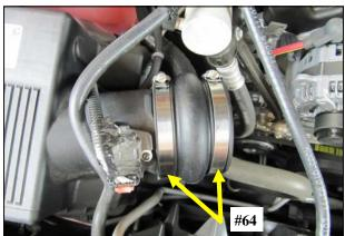
**5.** Slide the Hump Hose and #64 Clamps onto the factory air box. If you are installing an Airaid Jr. kit, install the Airaid Premium Filter at this time.
