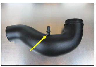
**3.** Install the Barbed Fitting into the Intake Tube as shown.
