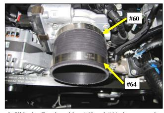
**6.** Slide the Coupler with a #60 and #64 clamp onto the throttle body as shown.
