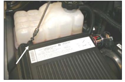
**7.** If you purchased the 200-996 kit, proceed to step # 9. If you purchased a Jr. Kit, remove 4 screws in the factory airbox with a #25 Torx bit, and remove the factory air filter. Proceed to step #8.
