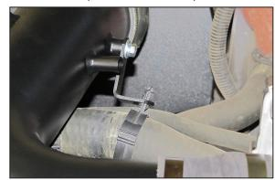
24. Install the upper radiator hose mount onto the mounting bracket installed onto the K&N® intake tube.
