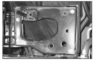
14. Remove the heat shield assembly and drill a 5/8"id hole through the marked location from step #13.
