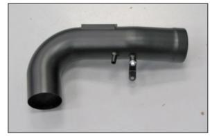
22. Install the "L" bracket (070812) onto the K&N® intake tube with the provided hardware as shown.
