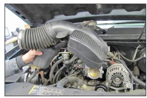
6. Loosen the hose clamps which secure stock intake tube to the throttle body and mass air sensor and then remove the intake tube from the vehicle.
