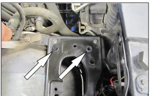
12. Remove the two air box mounting grommets shown.
