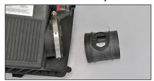
8. Loosen the hose clamp and remove the mass air sensor from the air cleaner as shown.
