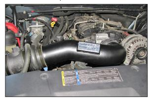
23. Install the K&N® intake tube into the silicone hose at the throttle body and mass air sensor and secure with the provided hose clamps.
