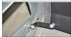
17. Secure the heat shield mounting bracket to the inner fender with the two fender washers and hardware as shown.
