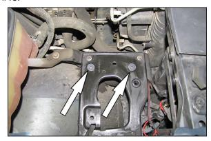
15. Install the two 5/16"inserted nuts into the air box mounting tray as shown.
