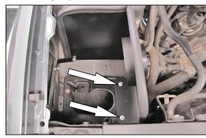
16. Install the heat shield assembly onto the air box-mounting tray and secure to the 5/16" inserted nuts with the provided hardware as shown.
