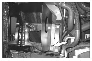
13. On vehicles not equipped with the front air box mounting grommet and hole, install the heat shield assembly as shown. Then use a marker to mark the mounting plate through the heat shield mounting hole.
