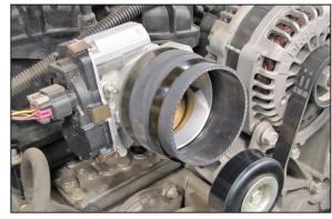
19. Install the silicone (08050) hose onto the throttle body and secure with the provided hose clamp.
