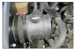
20. Install the mass air sensor assembly into the silicone hose on the filter adapter and secure with provided hose clamp.
