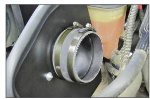
18. Install the silicone hose (08618) onto the filter adapter and secure with the provided hose clamp.
