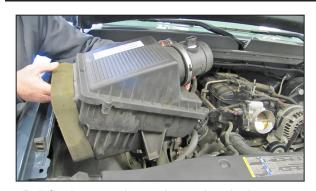
7. Pull firmly upwards to release the air cleaner assembly from the mounting tray grommets, and then remove the assembly as shown.
