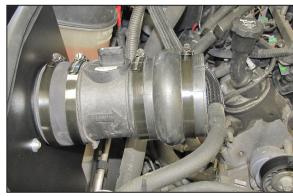
21. Install the silicone hump hose (08543) onto the mass air sensor and secure with the provided hose clamp as shown.
