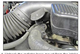
4. Unhook the radiator hose mount from the intake tube.
