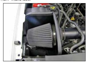
25. Install the K&N<sup>®</sup> air filter onto the filter adaptor and secure with the provided hose clamp.
