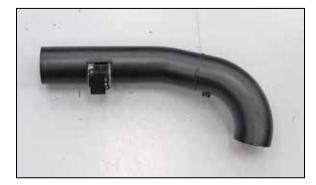
10. Install the mass air sensor into the K&N<sup>®</sup> intake tube and secure with the provided hardware.
