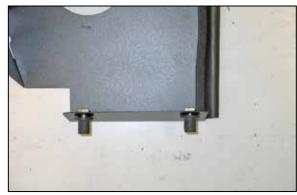
17. Install the reaming 5/16" inserted nut into the heat shield as shown.
