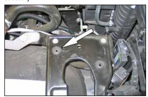
13. Remove the air box mounting grommet shown from the air box mounting plate.
