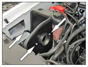
19. Secure the mounting bracket to the inner fender with the hardware provided. Then Install the filter adapter onto the heat shield and secure with the provided hardware.
