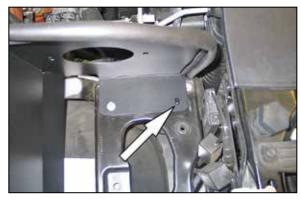
15. Set the heat shield assembly into position with the inserted nut installed into the air box mounting grommet location. Mark the heat shield mounting location to be drilled.
