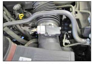
2. Disconnect the mass air electrical connection.
