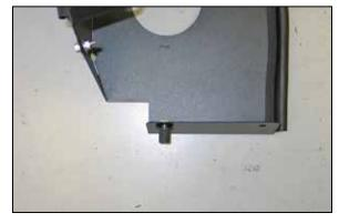
14. Secure the 5/16" inserted nut to the heat shield as shown.
