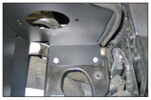
18. Reinstall the heat shield assembly onto the air box mounting plate and secure the two 5/16" bolts provided.
