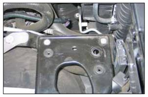
16. Remove the heat shield assembly and drill a 5/8" hole at the marked location.
