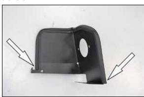
12. Install the provided edge trim onto the heat shield as shown. Note: Some trimming will be necessary.
