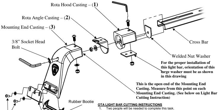
MATERIALS NEEDED: Hammer, center punch, pencil MATERIALS FURNISHED: One hardware pack, two end castings, four Rota castings, cross bar, instruction page.
