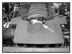
Step 4 Loosen the clamp at the throttle body and remove the factory plenum from the vehicle.
