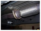
2. Remove the stock exhaust by unbolting it at the 2-bolt flange located in front of the muffler. Disengage the welded hangers from the OEM rubber grommets. Use WD-40 to aid in this process. Do not damage stock nuts and bolts or remove the rubber grommets as you will re-use them to mount your new system. Now, cut off tailpipe and remove system.
