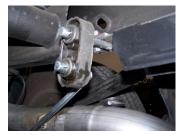
5. Next, remove your spare tire. Then install passenger side tailpipe hanger #J. You will see a  $1\frac{1}{2}$ " hole in the frame. Attach hanger to this hole and re-install factory grommet on hanger.
