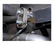
5. Next, remove your spare tire. Then install passenger side tailpipe hanger #J. You will see a 1½" hole in the frame. Attach hanger to this hole and re-install factory grommet on hanger.
