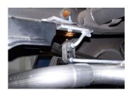
8. Now install driver side tailpipe hanger. Use same 1½" hole on the frame, but on the driver side. Install rubber grommet on hanger. Then install hanger from pipe into rubber grommet.
