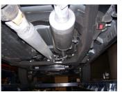
4. Install muffler #B onto headpipe  $1\frac{1}{2}$ "-2" with the louvers facing towards the converter. Use a jack stand to support the muffler. Use clamp #G to secure the muffler to the headpipe. Do not tighten. Muffler inlet is looking into the louvers.
