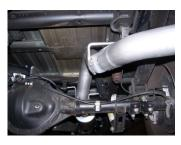
7. Slide exit pipe #D over tailpipe and secure with clamp #F. Do not tighten. Rotate exit pipe to best suit your vehicle.
