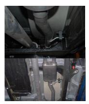
3.Next, install headpipe #A onto your factory flange. Insert welded gromment.
