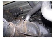
6. Install driver side tailpipe #D into muffler at least 1.5" to 2". This pipe will route over the axle and between the shock and spare tire. Use clamp #G to secure pipe to muffler. Do not tighten. Insert welded hangers into rubber grommet.
