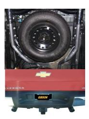
8. Install exit pipes #E onto tailpipes. Cut to your preferred length then use clamps to secure exit pipes to tailpipes. Install stainless steel tips. Clamp down. When you have everything in place, firmly tighten all bolts and clamps down securely. Use stainless steel cleaner and a Scotch Brite pad weekly to prevent tip from discoloration. Inspect all fasteners after 25-50 miles of operation and re-tighten as necessary.
