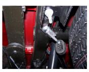
5. Install metal hanger #H into hole located approximately 16" from the rear of the frame. Use hardware kit #I, washer #M, and rubber grommet #J.
