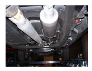
4. Install muffler #B onto headpipe  $1\frac{1}{2}$ "-2" with the louvers facing towards the converter. Use a jack stand to support the muffler. Use clamp #F to secure the muffler to the headpipe. Do not tighten. Muffler inlet is looking into the louvers.
