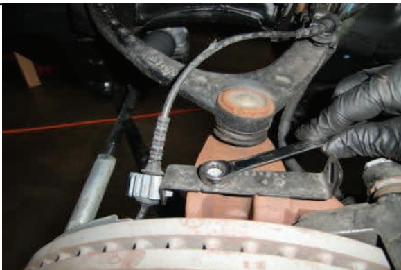
Disconnect ABS bracket on spindle
