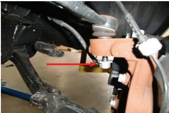
Leave nut attached as shown
