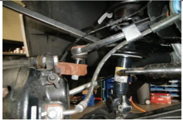
Use a pry bar to depress ball joint into spindle, attach nut
