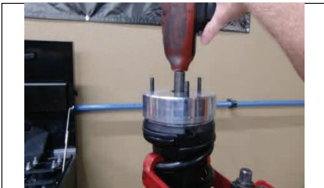
Use OE nut and tighten down to factory spec
