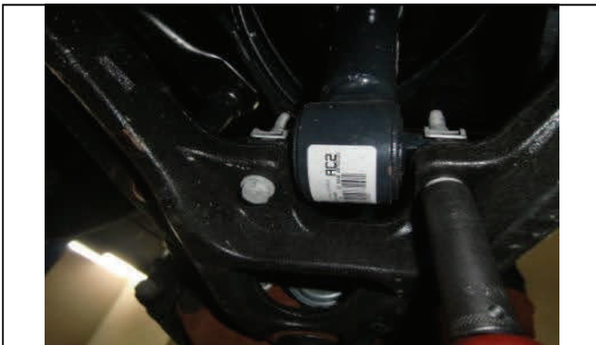
Remove lower strut mounting bolts
