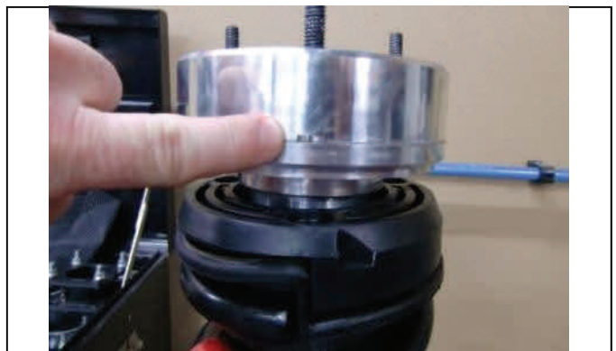
Note; Indexing mark and reposition onto strut assembly
