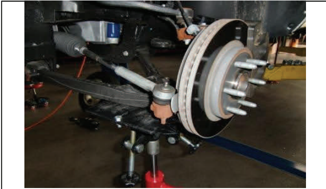
Support suspension with jack
