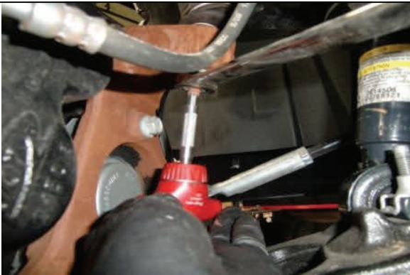
Tighten to spec, use allen wrench to hold ball joint stem
