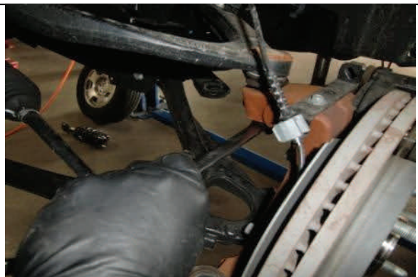
Loosen upper ball joint nut
