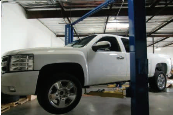
Raise and support vehicle by frame
