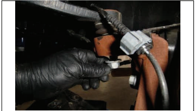
Now remove nut from ball joint
