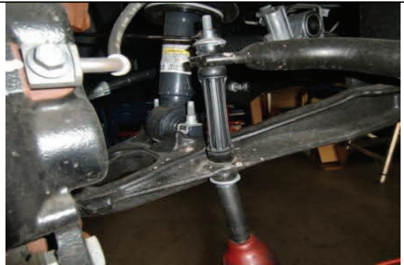
Reconnect sway bar end link and ABS/brake brackets
