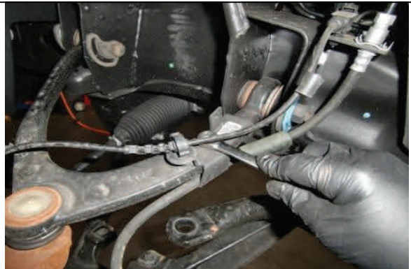
Disconnect ABS/brake line bracket on upper control arm
