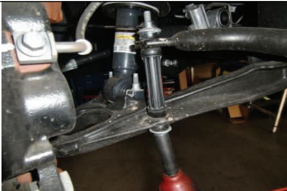
Disconnect sway bar end links
