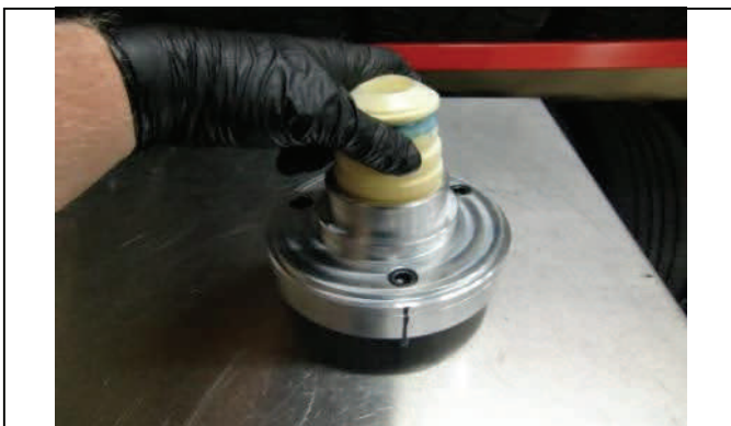
Install tight fitting OE bump stop into T6-3085
