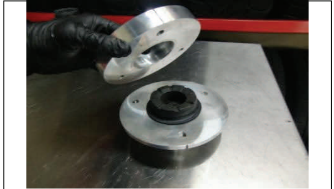
Place OE strut bushing between two halves
