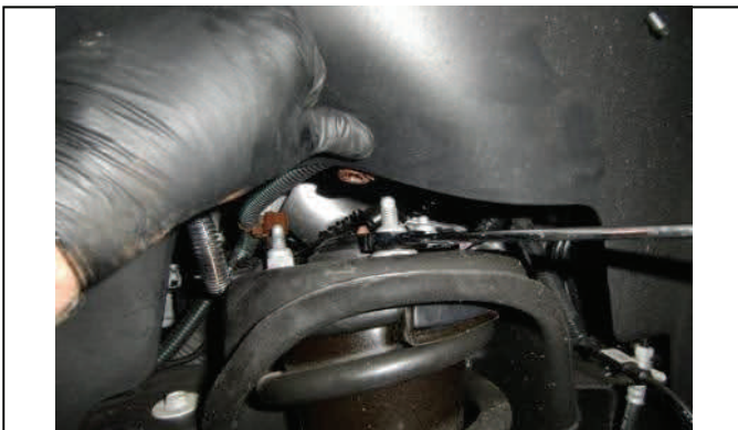
Remove upper strut mounting nuts
