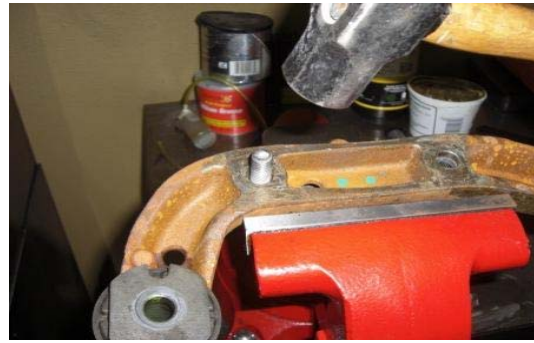
30. Secure in a vise and remove the mounting studs with hammer.
