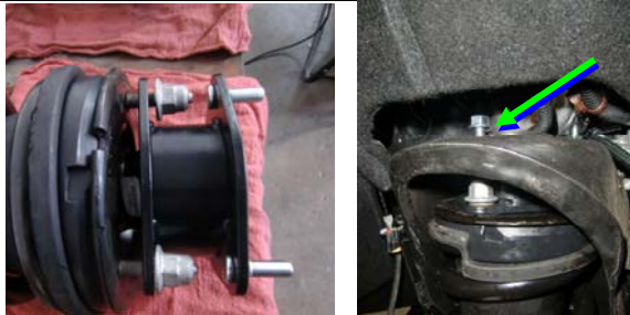
39. Place the new strut extension spacer onto the strut. Install strut with spacer leaving nuts loose.
