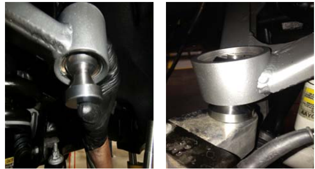
43-4. Insert the pin into the lower misalignment spacer.
