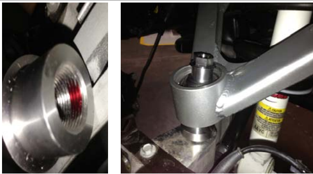
43-5. Lock-tite the upper misalignment spacer and install.
