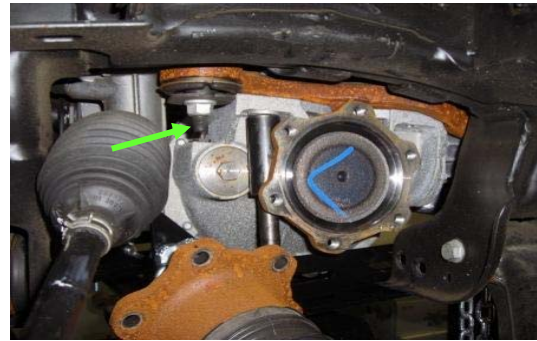
24. Remove the drivers side mounting bolts and unplug the vent line.
