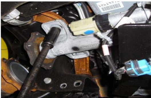
23. Support the differential with a jack and unbolt the passenger side.
