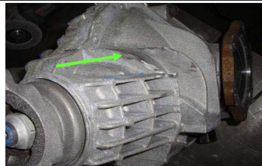
28. Use a grinder to remove the material marked previously.
