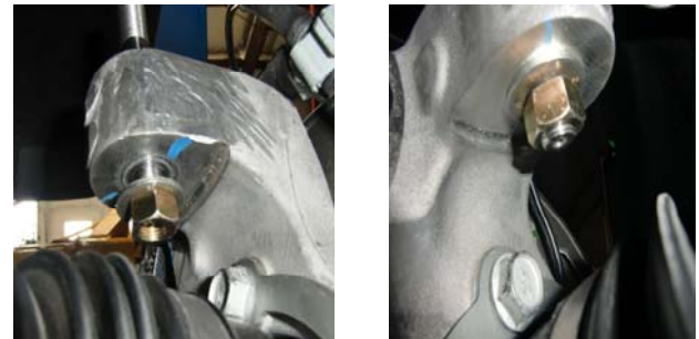
43-2. Add a washer and a standard nut . Tighten down to seat the
