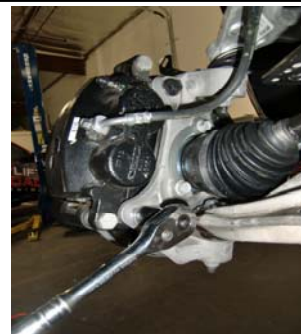
44-1. Re-attach brake calipers & torque to 145ft lbs.
