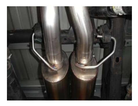
9. Install tail hanger using (2) 3" clamps.
