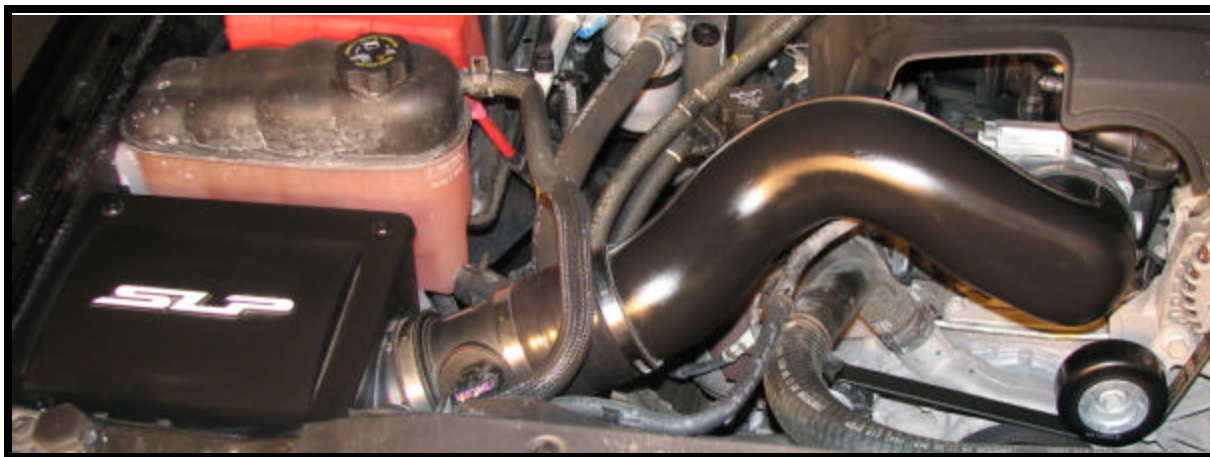
Photo 3: SLP Intake Tube Installed
