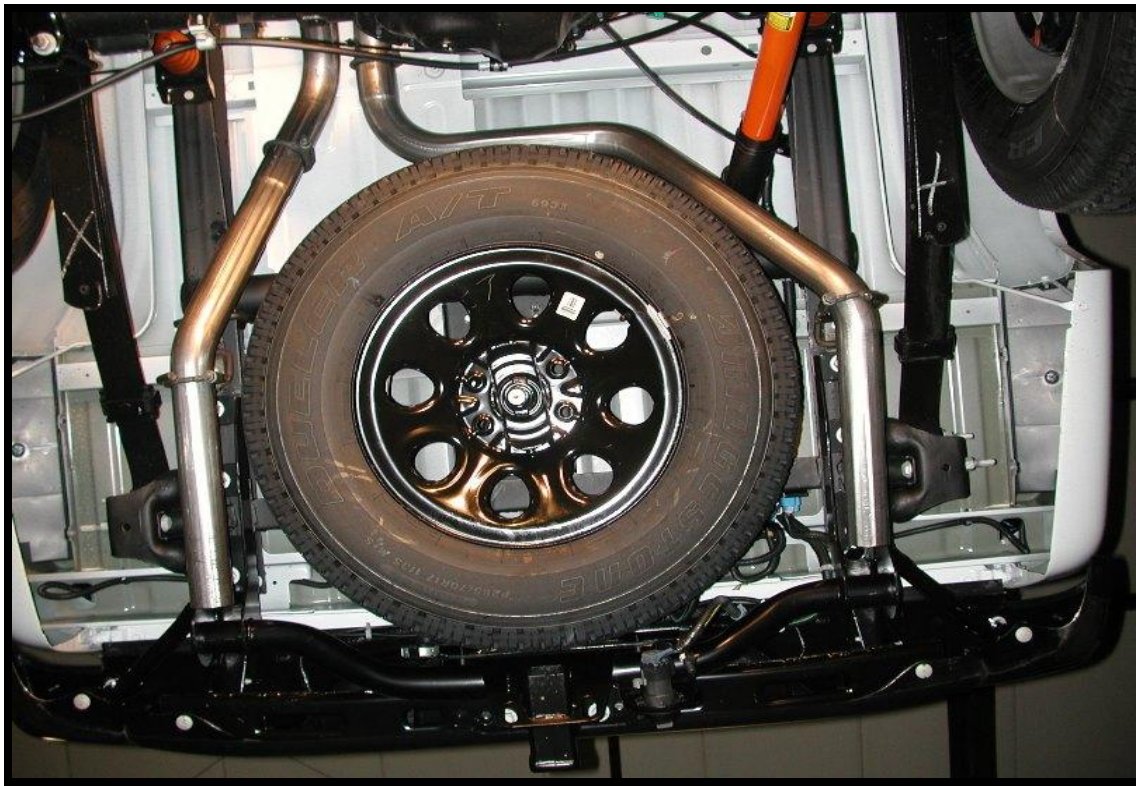
Figure 9: Drivers Side and Passengers Side Tailpipes Installed
