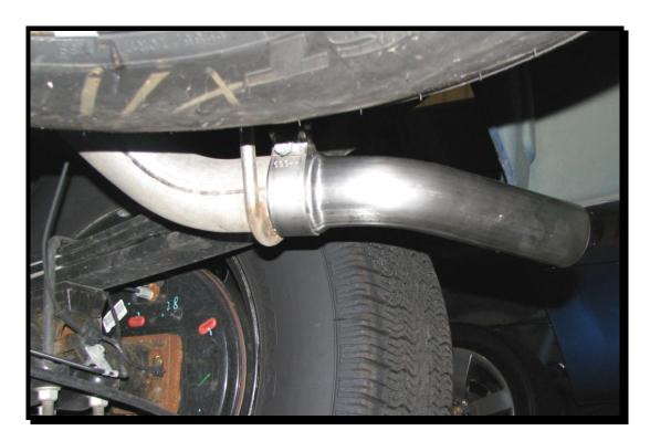
**Photo 1: Stock Pipe Removed from Vehicle**
