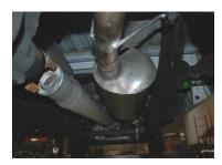
4. Install muffler #B onto headpipe 1½"-2" with the louvers facing towards the converter. Muffler outlet will be at the 9 o'clock position. Use a jack stand to support the
