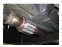
2. Remove the stock exhaust by unbolting it at the clamp Disengage the welded hangers from the OEM rubber grommets. Use WD-40 to aid in this process. Do not damage stock nuts and bolts or remove the rubber grommets as you will re-use them to mount your new system. Now, cut off tailpipe and remove system.
