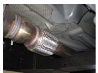
2. To remove stock exhaust, unclamp it at the ball flange behind the Y-pipe. Make sure to leave all rubber grommets in the factory location. **You will re-use stock clamp.** For easier removal of exhaust, cut behind the muffler. Use WD-40 to remove hangers from grommets.
