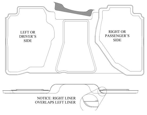
NOTE: IF YOUR TRUCK IS EQUIPPED WITH THE 40/20/40 FRONT BENCH SEAT, YOU WILL NEED TO TRIM AWAY A SECTION OF YOUR LINER. THIS IS EASILY DONE USING A UTILITY KNIFE OR PAIR OF HEAVY SHEARS. SIMPLY USE THE MOLDED IN GROOVE IN THE LINER AS YOUR TRIM GUIDE, REMOVING THE PORTION OF THE LINER ON THE "HUMP" PORTION OF THE LINER AS SHOWN ABOVE. MORE PHOTOS OF THE PART ARE ATTACHED ON THE BACK OF THIS PAGE.
