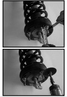
7. Locate the new front strut spacers. Install the new front strut spacers onto the strut and secure using the new 10 mm flange nuts. Make sure to use loctite and torque to **45 ft lbs.**
