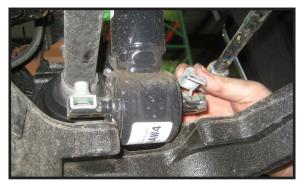
Working on the driver side upper strut mount, loosen the 3 nuts. It is not necessary to completely remove them. Repeat on passenger side
