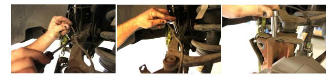
3. Remove ABS sensor from spindle and put it safely out of the way. Remove through bolt for sway bar end link and linkage.
