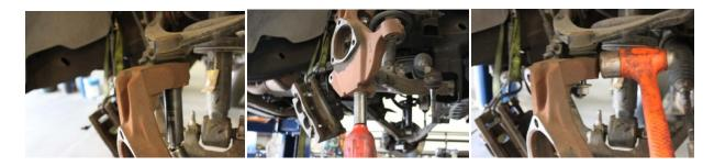
6. Support lower control arm and add pressure with a jack, then line up Maxtrac spindle with upper & lower ball joint, and loosely install nuts.
