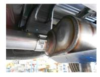
3) Place a supplied 3 <sup>1</sup>/<sub>2</sub>" clamp over the inlet of the muffler and then slide the inlet of muffler onto the back of the inlet pipe. Use a stand to support the muffler. Tighten the clamp just enough to hold in position.
