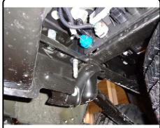
Install 1/2" carriage bolts, spacers, and flange nuts in remaining holes as shown. Torque all 1/2" hardware to 110 ft-lbs.
