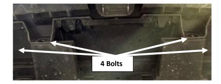
**Step 7:** Pull up and out (toward your body) on the top of the grill where the screws were to release the plastic tabs. Using your thumbs to push down on the bracket makes it easy.
