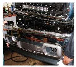
**Step 13:** Remove six bolts holding on OEM frame flanges to frame with 15mm socket. Set brackets aside.
