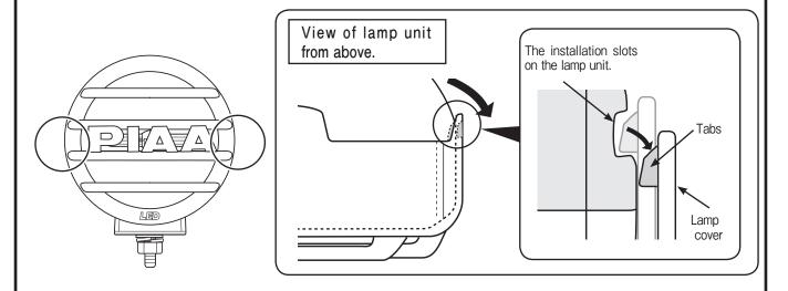
For installing the grill cover, first take the small tab on the upper edge of the cover and line it up with the slot on lamp unit and snap it in place. Then continue to snap the remaining tabs in place.
