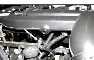
**2.** Pull the PCV breather line from the factory intake tube.
