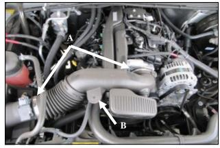
**3.A.**) Loosen the clamps securing the factory intake tube to the throttlebody and the airbox.
