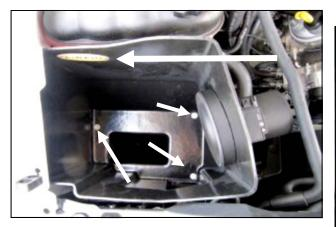
**10.** Install the **CAB** (#3) into the engine compartment and secure using three of the tray bolts from step **6.** Apply the Airaid Bubble decal inside of the Airbox as shown.
