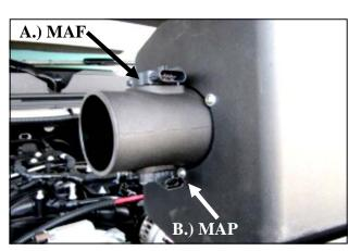
9. Install the Filter Adapter (#4) onto the Cold Air Box or CAB (#3) as shown using the three 1/4-20 Button Head Screws (#10) and 1/4" Flat Washers (#12).
