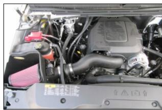
15. Reinstall the engine cover. Double check your work! Make sure there is no foreign material in the intake path. Make sure all clamps, hoses, bolts, and screws are tight. Double check the hood clearance. Reconnect the negative battery cable
