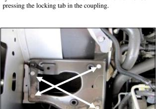
7. Remove the four tray bolts and the airbox mounting tray. Three of the bolts will be reused in step 9.
