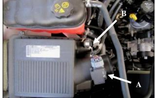
5. Disconnect the Mass Air Flow or MAF sensor (  $\bf A$  ) and the Manifold Absolute Pressure or MAP sensor (  $\bf B$  ) Remove the factory airbox from the vehicle.
