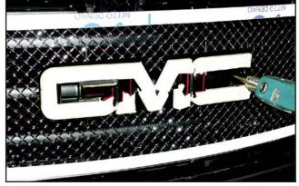
**16**. Use a 3/16" drill bit to drill through the marks made in the previous step.
