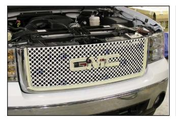
5. For "Denali" style grilles: Carefully align the "Denali" style grille over the factory grille and GMC emblem, making sure you do not damage the chrome plated GMC emblem or the emblem base. Use masking tape to hold the grille in place while aligning the mounting brackets.
