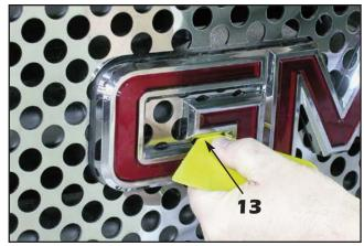
**13. NOTE:** E&G recommends slightly bending the bottome leg up for a tight fit against the plastic emblem base before installation. **"Denali" style grilles:** Once the double faced tape liner is removed, alilgn the "G" filler into place and use a plastic tool (such as a squeegee or body filler spreader) or a screwdriver wrapped in electrical tape to press the filler into place.
