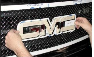
**15**. Align the stainless steel emblem surround into place and press firmly at the stud locations to make impressions into the factory plastic grille.
