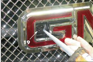
19. "Denali" style and Mesh grilles: Thoroughly clean the back of the stainless steel "G" filler and install the supplied double faced tape where shown.
