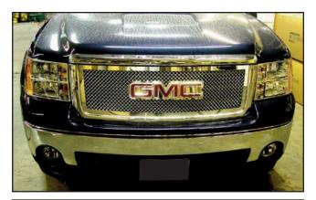
**21.** Reinstall the radiator support panel cover to finish.
