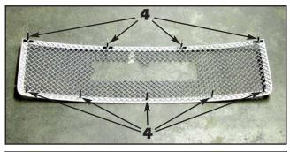
4. For Mesh Grilles: Align the mesh section onto the back of the mesh surround. Trim the closed ends from the preinstalled vinyl caps push them down over the studs. Trim the ends from seven (7) more vinyl caps and install an additional cap onto the studs across the bottom of the grille and another one half (1/2) sleeve onto the studs across the top of the grille prior to installation.
