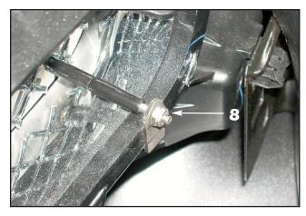
8. For Mesh grilles: Install the lower mounting tabs onto the studs at the bottom of the grille surround and install a #8-32 ESNA half nut onto each stud but do not completely tighten at this time. Leave the grille slightly loose to aid in masking tape removal outlined in Step 11.
