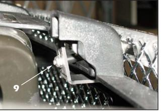
9. "Denali" and Mesh grilles: Align the upper mounting brackets so that they lock underneath the bottom edge of the factory grille fin. install a #8-32 ESNA half nut onto each stud but do not completely tighten at this time. Snug the nuts against the brackets to keep the brackets properly aligned (Mesh shown, "Denali" style grille same).
