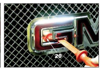
20. Once the double faced tape liner is removed, align the "G" filler into place and use a plastic tool or screwdriver wrapped in electrical tape to press the filler into place. Remove any silicone that may squeeze out around the filler.
