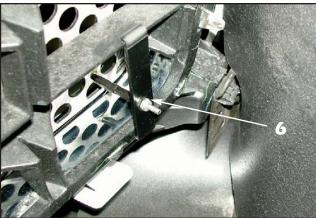
6. For "Denali" style grilles: Install the lower mounting brackets onto the studs at the bottom of the grille frame and install a #8-32 ESNA half nut onto each stud but do not completely tighten at this time. Leave the grille slightly loose to aid in masking tape removal out lined in Step 11.
