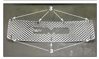
3. For "Denali" Style Grilles: Trim the closed ends from the preinstalled vinyl caps push them down over the studs. Trim the ends from seven (7) more vinyl caps and install the caps onto the mounting studs as well prior to installation.
