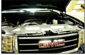
1. Remove the plastic radiator support panel cover by removing the plastic push pins.
