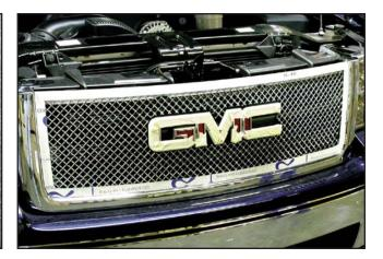
7. For Mesh grilles: Carefully align the mesh grille over the factory grille and GMC emblem, making sure you do not damage the chrome plated plastic GMC emblem or the emblem base. Use masking tape to hold the grille in place while aligning the mounting brackets and tabs.
