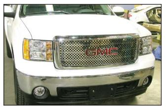
14. "Denali" style grille: reinstall the radiator support panel cover to finish. The remainder of the manual covers the final steps for the Mesh grille.
