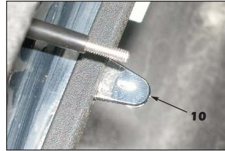
10. "Denali" and Mesh grilles: You must remove the factory center chrome tab before installing the lower center mounting bracket. The chrome tab will break off when you apply downward pressure onto it ("Denali" style shown, Mesh grille same). Once the tab has been removed, install the final lower mounting bracket.
