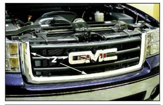
Thoroughly clean the factory grille and apply protective masking tape to the bottom of the chrome surround and to the top chrome surfaces of the GMC emblem.
