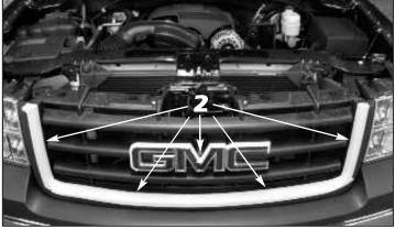
1. Open the hood and use a flat blade screwdriver to remove the factory push pins securing the top of the factory grille center section to the radiator support panel.
