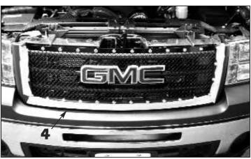
4. Carefully align the grille assembly into place and use wide masking tape to hold the grille in place during the hardware installa-
