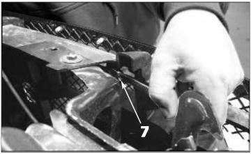
**7.** Use the u-shaped grille retainers on the center upper mounting studs. Due to their location, it will be necessary to use a 9mm wrench to tighten the #8-32 ESNA half nut. Tighten only until the studs are flush with the back of the ESNA nut.
