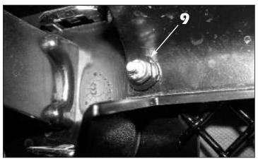
**9**. Realign the emblem surround and install the supplied small back plastic washers and the #8-32 ESNA half nuts and tighten to secure the emblem surround.
