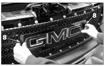
8. Align the GMC emblem surround in place and press firmly enough to indent the stud location on the factory grille center bar. Use a 1/4" drill bit to drill through the marks made (not shown).
