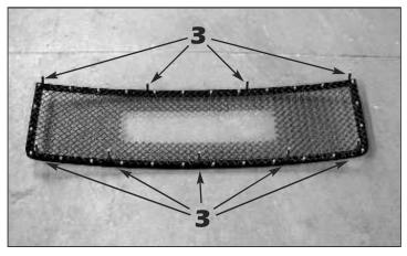
3. Align the mesh section onto the back of the E-Power surround. Trim the ends from the supplied #8 x 1-1/4" black cap plugs and the #8 x 3/4" black cap plugs and install them over all mounting studs up so that only 3/8" of threads are exposed.
