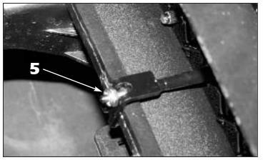
**5.** Install the lower u-shaped grille retainers across the bottom of the grille using the supplied #8-32 ESNA half nuts. To install the center bracket, you must break off the small mounting tab (not shown).
