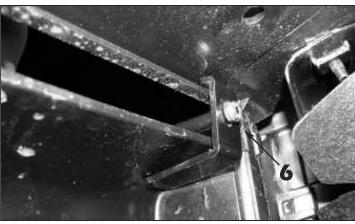
**6.** Install the upper outer grille retainers using the supplied #8-32 ESNA half nuts (as shown).
