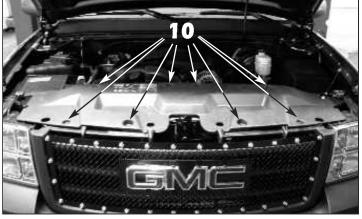
**10**. Align the factory radiator support panel back into place and install the plastic push pins and close the hood to finish the installation.
