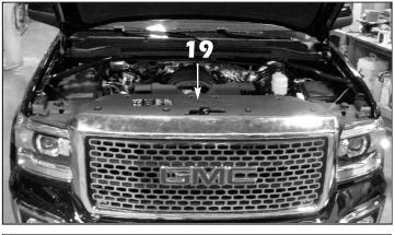
**19.** Align the factory radiator support panel back into place and install the plastic push pins and close the hood to finish the installation.
