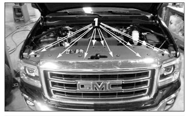
**1**. Open the hood and use a flat blade screwdriver to remove the factory push pins securing the top of the factory grille center section to the radiator support panel.
