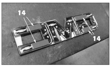
**14.** For customers requesting emblem reinstallation: Cut the supplied .090" x 1" double faced tape and the .045" x 1" double faced tape into 2-1/2" long strips and install the strips where shown on the back of the emblem. Stack 2 strips of the .090" thick tape with one strip of the .045" thick tape at each of the four locations.
