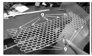
**9**. Trim the ends from the supplied black cap plugs and install them over the mounting studs on the back of the E&G grille.
