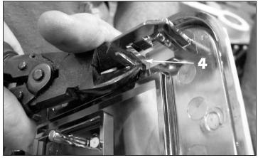
**4.** For customers reduces the emblem reinstallation: Carefully cut the factory mounting tabs from the back of the factory emblem.
