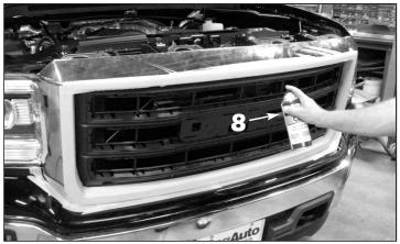
**8**. Apply flat or semi-gloss black paint the any areas on the factory grille that were stressed during the chrome moulding removal. The stressed plastic will appear light gray or white.
