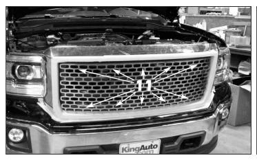
**11.** Install the E&G grille over the factory grille making sure all mounting studs pass through the openings in the factory grille.
