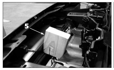
**5**. Cut a 4" section of 2 x 4, lift up and pull forward on the upper portion of the factory grille and place the 2 x 4 section where shown to allow access for hardware installation.
