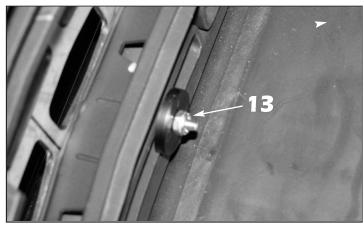
**13.** Install the supplied large black plastic washers across the bottom of the grille using the supplied #8-32 ESNA half nuts.
