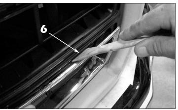
**6**. Remove the factory chrome inserts from the factory grille. Use a plastic clip removal tool to start the removal process.
