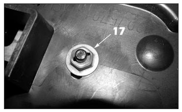
**17.** Install the supplied speed nuts onto the factory alignment pins and once started, turn the nut an additional 1/4 to 1/2 turn to secure.
