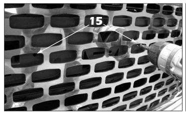
15. For customers reauestina emblem reinstallation: Locate the existing alignment pin holes for the factory emblem. Use a 1/4" drill bit to drill new holes directly below the factory holes.
