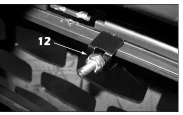
Install the grille upper mounting brackets using the supplied #8-32 ESNA half nuts (as shown) to all five upper mounting studs. Tighten until the E&G grille is snug against the factory grille.
