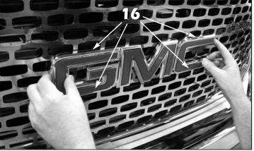
**16.** For customers requesting emblem reinstallation: Peel off the double faced tape backing from the tape installed in step 14. Align the factory emblem with the holes drilled in the previous step and press firmly enough to set the tape.
