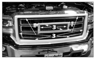
**3**. Apply masking tape around the factory GMC emblem and use a plastic clip removal tool to pry the emblem around the perimeter until the emblem releases (not shown). Once the emblem has been removed, apply masking tape to the factory chrome surround.
