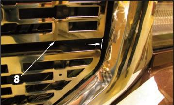
8. Install the upper grille center section using the same procedure outlined in Steps 6 and 7. Make sure that the edges of the grille align with one another. You can use a small secton of wood or plastic and insert it into any of the grille openings and tap the wood or plastic with a mallet to adjust the side to side gap (alignment).
