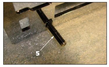
**5**. Paint all of the lower studs on all three grille sections with black paint to help conceal them once the grille sections are installed.
