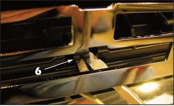
**6**. Begin aligning the upper grille bottom section first. Align the center two studs where the factory retaining clips are located. Insert a small flat blade screwdriver to pry the tab away from the stud and press in on the grille to begin seating the studs. Work from the center out, alternating from bottom to top studs.
