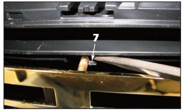
7. Continue aligning the studs with the retaining clips. Move the clips as needed to press the grille tightly against the factory insert. Make sure that once the upper grille bottom section is pressed into place that it is perfectly centered inside the factory chrome surround.
