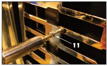
Install the supplied #6 x 3/4" Torx pin head screws to secure the outer edges of the E&G grilles and finish the installation. Do not overtighten or you could indent the grilles at the screw locations or strip out the holes in the factory plastic grille.
