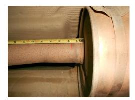
2) Support the muffler and muffler inlet pipe with a stand. At the front of the factory muffler, measure out 1.50" and make a mark on the pipe. Using a hacksaw or sawsall, cut the inlet pipe on this mark. Separate the wire hangers at the back of the muffler and on the tailpipe from the rubber mounts on the vehicle. Remove the muffler and tailpipe from the vehicle. Use a file or die grinder to remove any burrs from the inlet pipe.
