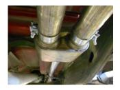
5) Place two of the supplied 3" clamps over the right and left outlets of the muffler. Place right tailpipe **#26431S** into position over the rear axle, and slide into the right muffler outlet. Connect the two hangers on the pipe to the rubber mounts on the vehicle. Pipe should be approximately 3/4" away from the shock when adjusted.
