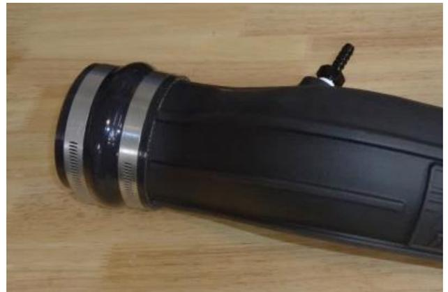
22. Slip two hose clamps (8) onto the other 3 $\frac{3}{4}$ " - 4" coupler (14). Install the 4" end of the coupler on the Filter end of the intake tube, and snug (but do not yet tighten) the hose clamps.
