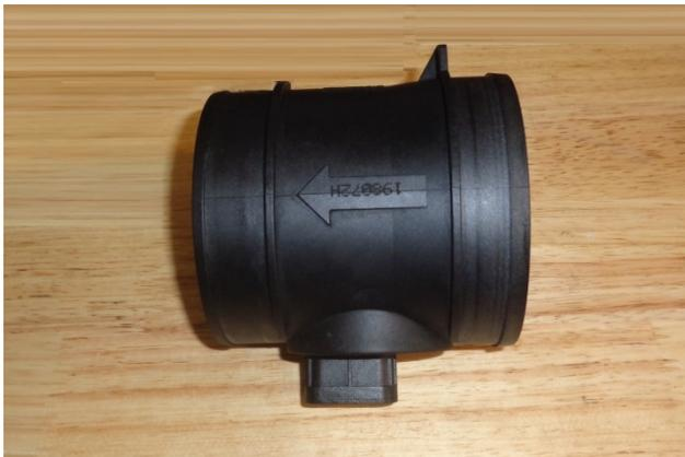
13. Remove the MAF sensor from the airbox.
