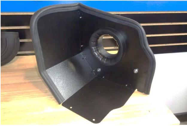
18. Attach gasket (4) to heat shield as shown. Starting at one end, firmly press the gasket onto the edge, gradually working around the heat shield. When you arrive at the ending point, use metal-cutting shears to trim the gasket to length.
