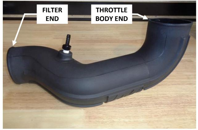
21. Apply 2 wraps of nylon thread tape to threads of 3/8" barbed fitting (9), and install it in the intake tube (13). Note the Filter and Throttle Body ends of the tube (for the next two steps).
