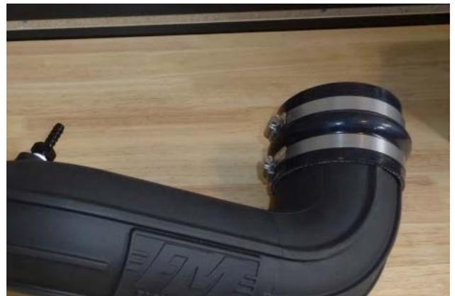
23. Slip the last two hose clamps (8) onto the 4" coupler (12), then install the coupler on the throttle-body end of the intake tube. Snug (but do not yet tighten) the clamps.
