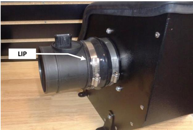
19. Slip two hose clamps (8) onto a 3 $\frac{3}{4}$ " - 4" coupler (14). Push the coupler's 4" end onto the air filter adapter, all the way against the heat shield, and tighten the clamp. Orient the MAF sensor so that the airflow arrow points away from the coupler, and push the sensor fully into the coupler, so that its lip touches the coupler, then tighten the clamp.
