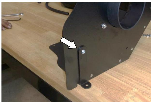
16. Attach long bracket (16) to heat shield using 1/4-20 screw (15) (against the bracket) and nut (21), lock washer (20) and flat washer (19) (against the heat shield). Do not fully tighten hardware at this time.
