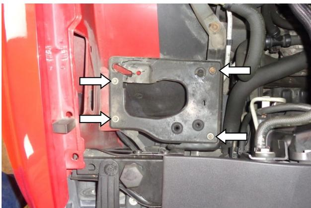
14. Remove the airbox shelf mount bolts, and remove the shelf. Retain the bolts for installation of the heat shield at Step 20. **NOTE: During removal of airbox shelf mount bolts, if there are any differences in bolt length, note each bolt's location, in order to maintain proper hardware clearance at reinstallation.**
