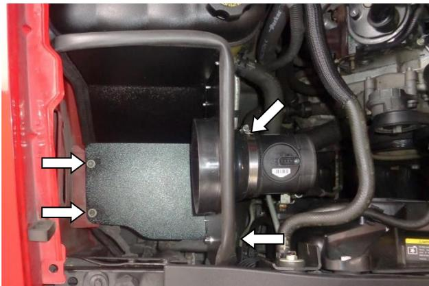
20. Place the assembled heat shield in the vehicle, and secure it with the 4 bolts retained at Step 13. **NOTE: To maintain hardware clearances, use the correct length bolt at each location (as noted in Step 14).** Then tighten the heat shield bracket screws.
