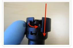
Disconnect the intake tube from the air cleaner assembly. Then remove the intake from the vehicle.
