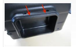
**13.** Install the Air box assembly using the supplied M6-1.0x10mm Screws (T) and 6mm Washers (U) in the two holes closest to the fender and the 2 longer OE screws in the remaining two holes.
