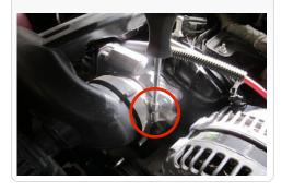
9. Remove the air cleaner box from the vehicle by carefully pulling it up out of the factory grommets.
