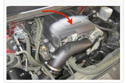
22. Push the Silicone Breather Hose (Q) over the Hose Barb (P) on the Intake tube. Then push the other end onto the valve cover vent line. Trim hose to desired fit if necessary. Hose should not be resting on other parts
