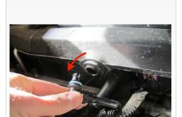
3. Disconnect the crank case vent line from
