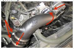
24. Re-install the engine cover. Inspect your installation, make sure the kit is properly positioned and all fasteners are secure.
