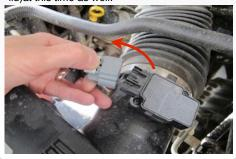
8. Using a flat blade screwdriver, remove the intake tube from the push pin located on the coolant tube. Then remove the intake from the vehicle.
