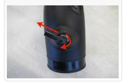
**11.** For those concerned about minimal engine heat; install the Air Inlet Plug (A) into the bottom of the Air Box (B) by pushing it down until the bead catches the lip as shown below. For those seeking additional air flow, set the Air Inlet Plug aside. (See page 3 for more info and test results)
