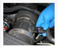
4. Pull the crankcase breather line from the OE intake tube and from the engine and remove
