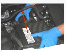
8. Loosen the hose clamp on the OE air box and remove the MAF sensor.
