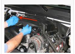
3. Disconnect the electrical connection to the MAF sensor at the OE air box.
