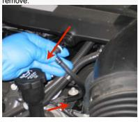
5. Pry the OE plastic radiator hose binder from the intake tube
