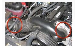
7. Slide the OE air box towards the engine while pulling up, to remove from vehicle.
