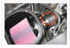
13. Place the S&B hump adapter (M) over the S&B tube (O), slide on until rib on tube is captured by the groove in the adapter. Then secure with #60 hose clamp (K).
