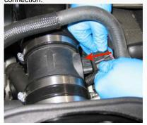
17. Install the 3/8" crankcase vent hose (Q) from the engine over the radiator hose to the S&B Intake tube (O), secure both ends
