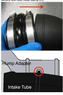
14. Install the S&B step adapter (P) to S&B tube (O) as shown, secure the #72 hose clamp (R).
