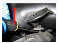
6. Loosen the hose clamp at the throttle body and at the MAF sensor, remove the OE intake tube from the engine
