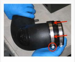
15. Install the S&B tube (O). Place the hump adapter end over the MAF and secure the #60 hose clamp. Then place the other end with the step adapter (P) over the throttle
