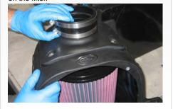
11. Remove the OE bolt located on top of the core support between the fender and hood bumper, Install the S&B air box (H) align prongs to OE grommets and secure the box using the Tapered Allen Head Bolt (F) & Thin SS washer (G) supplied.
