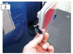
Attach one of the support bracket to the alignment pin located behind the taillight, Hold the support bracket in place as you re-install the taillight back onto the vehicle.
