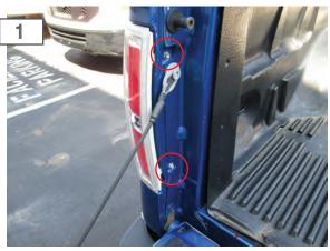
Start by opening the tail gate to access the two (2) factory bolts that hold the tail light in place. Remove bolts (these will be reused).
