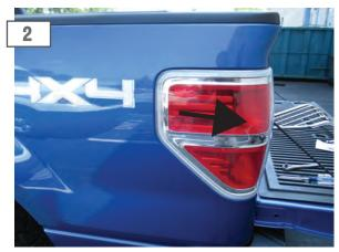
Apply firm pressure on the tail lights. There is one(1) clips that holds the front of the tail light in place. This clip will pop out with pressure. \*\*Note: I used the palm of my hand to dislog the clip.
