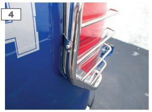
Secure the taillight with the two factory bolts. Do not tighten at this time.
