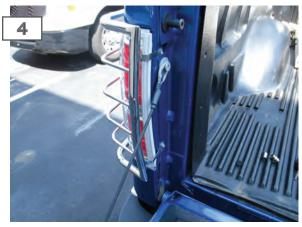
Attach the taillight guard to the support bracket using the supplied hardware.
